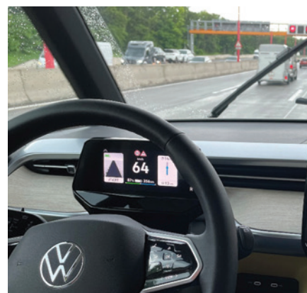
V2I Dashboard Alert of Speed Limit and Road Condition on A23 Motorway in Vienna, Austria.
