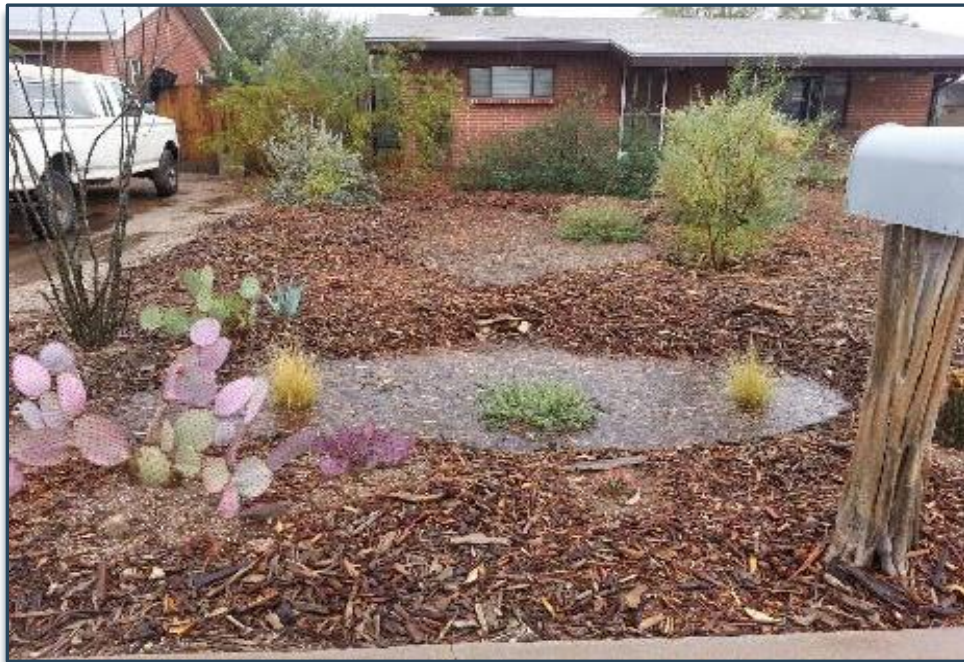
Photograph 7-12 Rain gardens, harvesting water from the roof and the street, harvest large volumes of water for native shade trees, grass and shrub irrigation.
